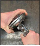
Holding both the thermometer face and the adjustable bracket, rotate the thermometer face to the desired position. No more than minimum force should be required.
