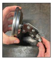
Set the thermometer face to the required angle. Retighten the screws.
